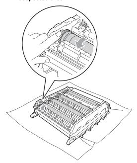
When you have found the mark on the drum that matches the drum dot check sheet, wipe the surface of the drum gently with a cotton swab until the mark on the surface comes off.
